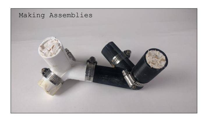
Show how molds connect to reproduce a design assemblies are made using stainless steel clamps to provide stong, adjustable uniform pressure
